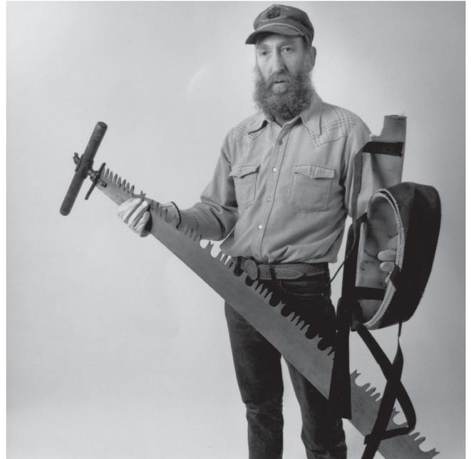
Figure 7—The sawguard is rolled and ready to be applied to the saw.
