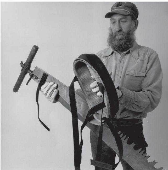
Figure 8—Unrolling the sawguard along the saw's cutters.
