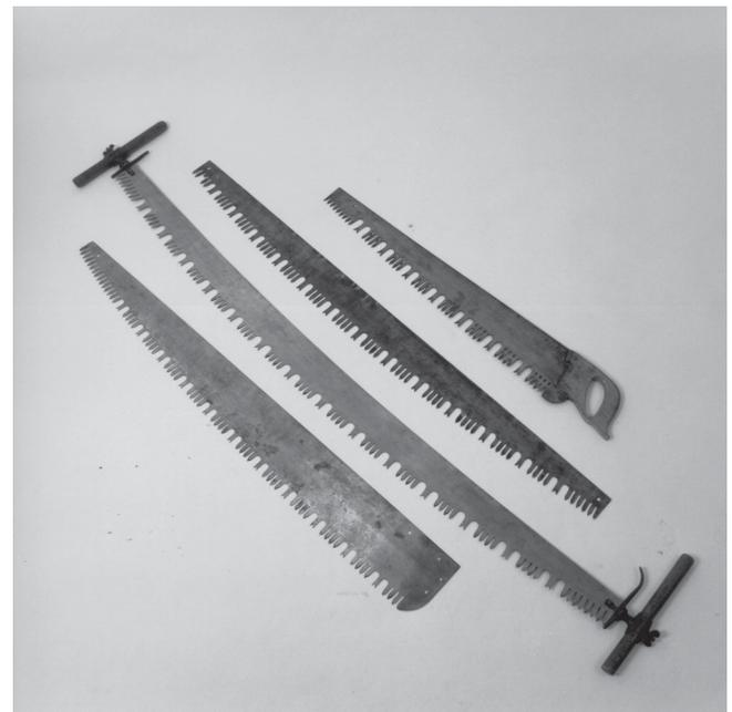
Figure 1—Several different styles and lengths of crosscut saws.
